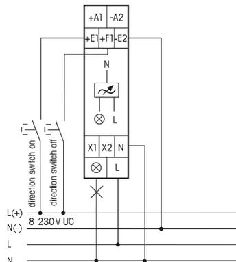
**Function 'Udo'** = Same as universal dimmer switch EUD but also comprising setting for a time delay from 1 to 99 minutes. Switch-off early warning at the end by dimming is selectable and adjustable from 1 to 3 minutes. The two central inputs are active.
