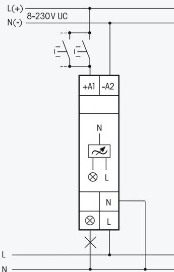
**Mixing of L loads and C loads** is possible with dimmer switches **EUD12Z** (description page B2) and **EUD12D** (page B3) in connection with capacity enhancer **LUD12** (page B5).
